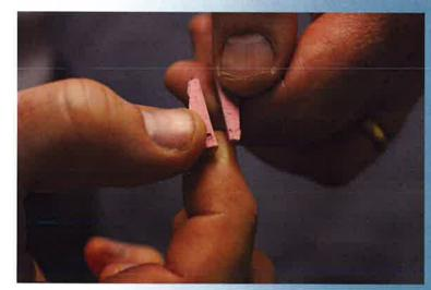
The cones will break along the thin center section
